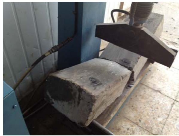
Fig. 1: Ultrasonic pulse velocity test method
